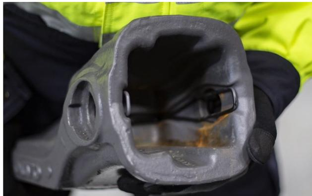
If you remove a tooth maybe for changing position, always check the retainer so it's not bended or damaged.
