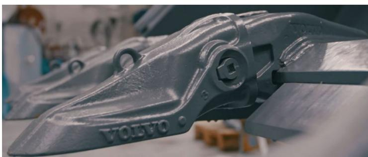
If you plan to place the flange on the pin on the right-hand side at the tooth, start install the teeth from the left. That will give more space for the tool.
