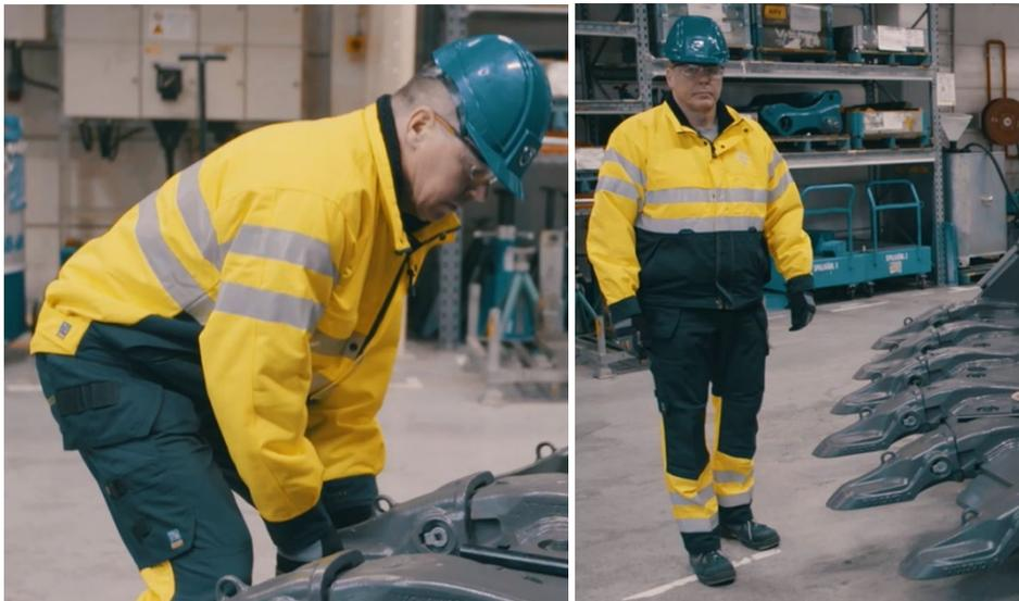
Check so the tooth is secured to the adapter – job done.
