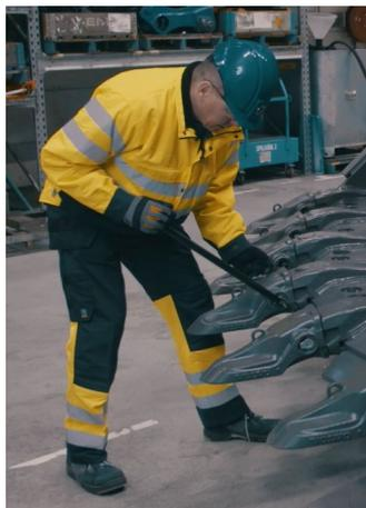
Take the tool and put it into the pin socket.
