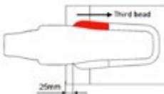
8. Repeat this sequence (steps 5, 6 and 7) three times. Vary the lengths of the beads slightly so that the start/stop positions are not at exactly the same location.
