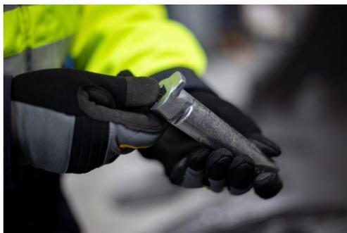
Check the pin so it is not bended or damaged.
