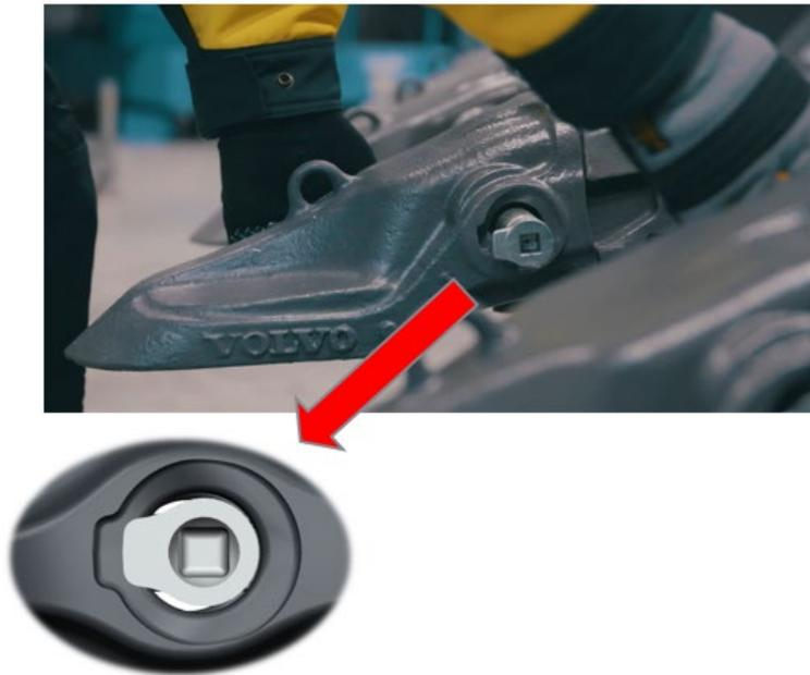
Place the locking pin in position and attach the tool. Check so the pin flange is align with the adapter. You can attach the pin from both left and the right side.
