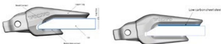
Alternatively, the upper leg adapter may be built up by welding to acceptable dimensions in the following manner:
