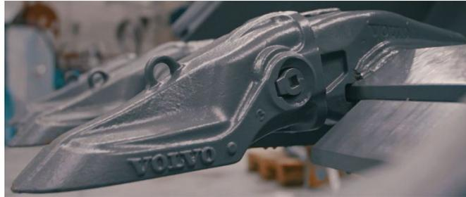
If the flange on the pin is located on the right-hand side at the tooth, start remove the teeth from the right.
