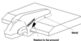
19. Grinding shall produce a smooth surface free of roughness and unevenness associated with the weld beads. The toes of the welds shall merge smoothly with the lip and the adapter with a minimum radius of 4mm (0.16 in). Grinding shall be done using high speed electric or pneumatic grinders with grinding wheels no larger than 50mm (2.00 in) in diameter.
