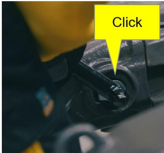
When a CLICK sounds, the pin is mounted correctly.
