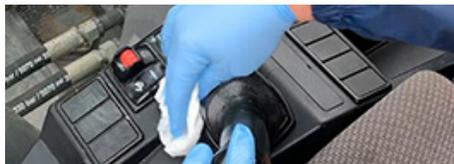
**4.** Be careful when cleaning electronic consoles and display interfaces. An EPA-approved, contactless product may leave a film when it dries, but it's not necessary to wipe it off once you achieve full coverage. If necessary on electronics, use a soft cloth or microfiber cloth and discard after use.
