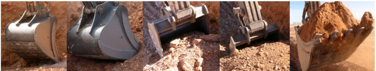
The Volvo bucket makes penetration, then is pulled into the material and fills smoothly. After filling, the bucket cradles the material and is ready for dumping.
