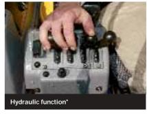
The hydraulic system in the L50D is prepared for installation of a third hydraulic function. The separate third hydraulic function, with its control lever and additional lines, can easily be installed to further increase the machine's flexibility.
