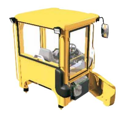
the left of the steering wheel and on the hydraulic console to the right. With Comfort Drive Control (CDC)\*, the operator can operate steering, forward, reverse and kick-down with controls on the left armrest. At any time, the operator can switch between steering with the steering wheel and CDC, which helps to minimize tiring and repetitive movements. This gives the operator the possibility to vary operating modes, thus combatting fatigue and static muscle strain.
