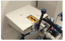
HYDROSTATIC PUMP CONTROL The hydrostatic drive on the HT-540 allows variable volume flow through the robust 2" material pump, providing unparalleled efficiency to fit any size application.
