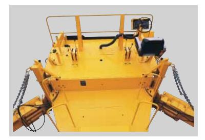
Control functions located on the operator's console include main power, starter throttle, horn, conveyor speed, shuttle and discharge direction, strike-off lift and lateral movement, hopper lip position and front and rear steering.
