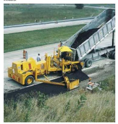
When shipping or traveling on the job, the strike-off can be swung flush with the side of the machine to limit overall width to 11'11" (3.63 m). A second strike-off assembly can be added to the opposite side of the machine to virtually eliminate the changeover time required in operations where frequent changes in right/left side material discharge are necessary.
