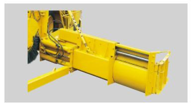
3' (914 mm) Hydraulic Strike-Off Extensions: A hydraulically extendible strike-off extension (left side or right side) that can be mounted on the outer end of either the standard 3' (914 mm) or 6' (1829 mm) contoured strike-off sections to provide additional "on-the-go" variable operating width flexibility in conjunction with the standard 2' to 3' (610 mm-914 mm) telescoping sections.
