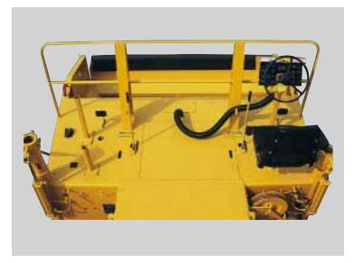
Control functions located on the operator's console include main power, starter throttle, horn, conveyor speed, shuttle and discharge direction, strike-off lift and lateral movement, hopper lip position, steering and parking brake.
