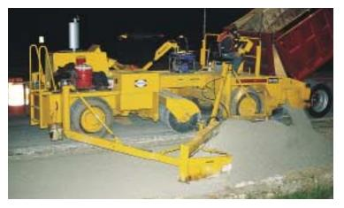
**Truck Hitch:** Two bearing equipped push rollers mounted on an oscillating frame with electric/hydraulic actuated, roller equipped clamp arms; quickly grips and secures a truck in proper attitude for unloading material into the machine's hopper; automatically compensates for both minor lateral and directional misalignment of truck with road widener with no exposed secondary slide mechanisms.
