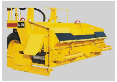
**Power Adjustable Front Hopper Lip:** Hydraulically adjustable front hopper chute with Tivar® polymer retaining lip [8<sup>5</sup>/<sub>8</sub>" (219 mm) high at the outer ends, 5<sup>5</sup>/<sub>8</sub>" (143 mm) high in the center] is infinitely adjustable in height up to a maximum of 7" (178 mm) to accommodate varying truck bed heights and reduce spillage during the dump cycle.
