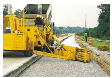
When shipping or traveling on the job, the strike-off can be swung flush with the side of the machine to limit overall width to 10'10" (3.30 m). A second strike-off assembly can be added to the opposite side of the machine to virtually eliminate the changeover time required in operations where frequent changes in right/left side material discharge are necessary.
