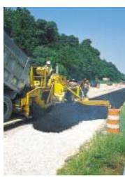
The conveyor will discharge material from either side of the machine. Discharge direction, left or right, is controlled with an electrical switch on the operator's console. Note that to accommodate opposite side discharge, it is necessary to transfer the strike-off assembly, hopper confining chutes, operator's console and seat to the opposite side of the machine. Unless otherwise specified, all RW-100A Road Wideners are shipped from the factory set-up for right side discharge.
