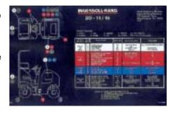
lifts easily, giving ground-level access to the engine, radiator, battery, and filters. Colorcoded service charts show detailed checkpoint locations, service intervals and proper lubricants.
