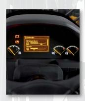
Refined computer programming will alert operators when regeneration needs to occur.
