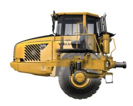
The reliable three-point suspension consists of heavy duty components.
