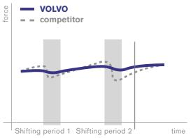
The electronically controlled transmission allows the Volvo haulers to maintain high and constant speed during shifting.
