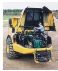
Access to the whole engine compartment is superb thanks to the new engine hood. An access ladder incorporated in the front grille makes it very easy to reach the various service points.
