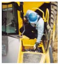
The batteries are easily accessed outside the cab.
