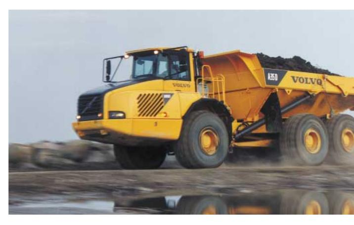
The front axle's sturdy rubber suspension with shock absorbers means the hauler can maintain high average speeds while maintaning operator comfort and minimizing mechanical wear. The bogic design means that each pair of wheels can move independently to maintain ground contact. This lets the body stay practically level over rough ground while the frame undergoes less stress.
