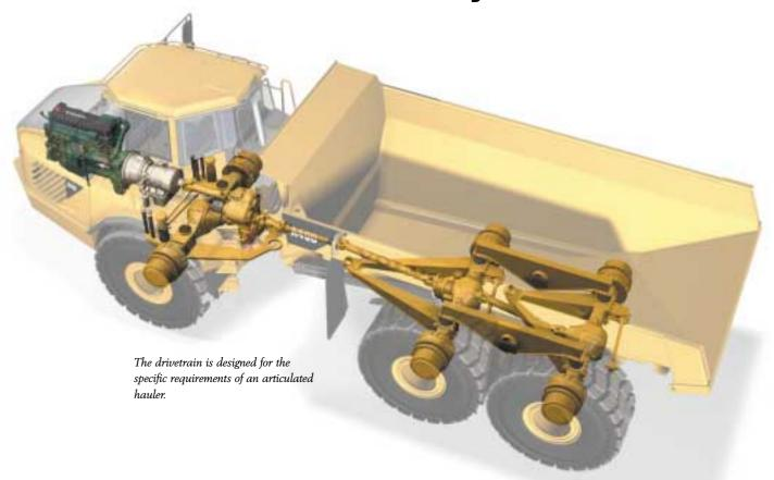
The reason that the articulated hauler is so successful is that the drivetrain is fine-tuned and optimized for its job. Volvo's articulated haulers have always been characterized by a drivetrain that is designed for the specific requirements of an articulated hauler.
