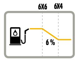
Always operating with the correct drive combination reduces fuel consumption by up to six percent.
