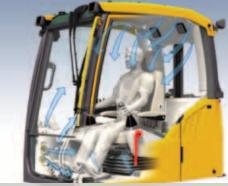
Industry's highest heating/cooling capacity with 14 vents.
