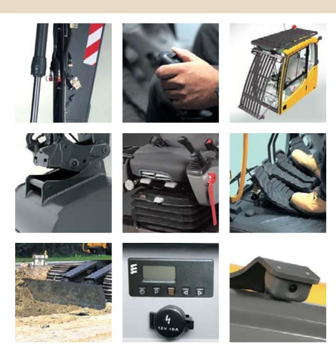
Hydraulic kits Hydraulic quick fit Dozer blade Wrist control joysticks - proportional control
