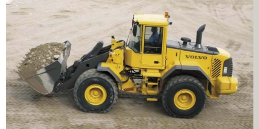
Boom Suspension System (BSS)\* BSS utilizes gas/oil accumulators connected to the lift cylinders to absorb shocks and smooth out rough roads for faster cycle times, less spillage and increased operator comfort.
