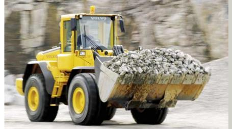
Boom Suspension System (BSS)\* BSS utilizes gas/oil accumulators connected to the lift cylinders to absorb shocks and smooth out rough roads for faster cycle times, less spillage and increased operator comfort.
