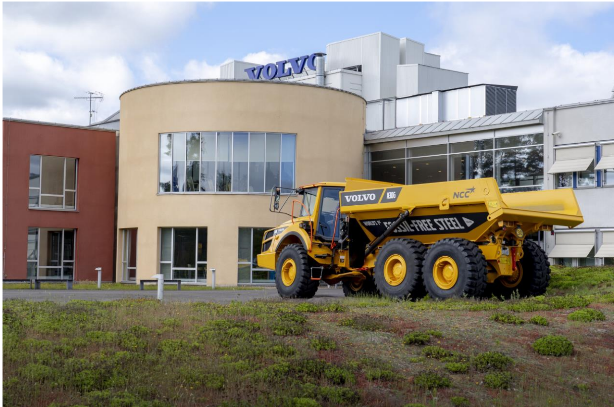
The A30G articulated hauler made from fossil-free steel was built at Braås
