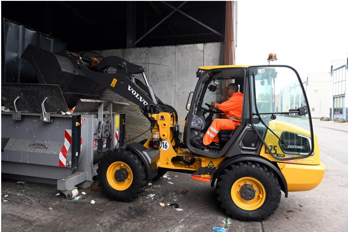
The L25 Electric wheel loader transports waste from 26,000 garbage bins in the city into compacting containers
