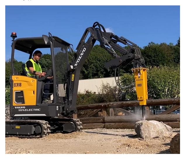
The new hydraulic breakers, HB01 and HB02, are designed to work in harmony with Volvo CE's smallest compact excavators, delivering robust yet lightweight power ideal for urban and indoor projects. The HB01 is a brand-new class of hydraulic breaker, while the HB02 is an updated version of its predecessor, providing improved specifications.
